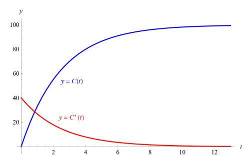
C' tells us how fast the battery is charging per hour at any time t.
